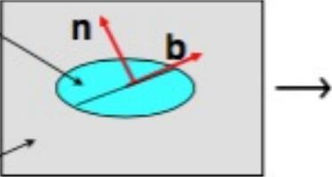
Solve stress equilibrium equation for inclusion in the homogeneous medium  $\longrightarrow \sigma_{ij,j} = \frac{\partial \sigma_{i1}}{\partial x_1} + \frac{\partial \sigma_{i2}}{\partial x_2} + \frac{\partial \sigma_{i3}}{\partial x_3} = 0$
