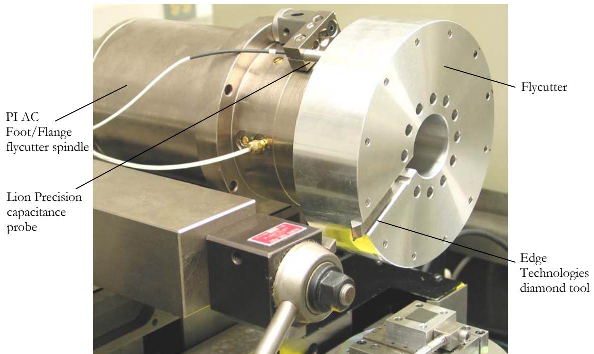
Figure 4.4: Close-up view of the AC foot/flange flycutter spindle mounted on the x-axis.
