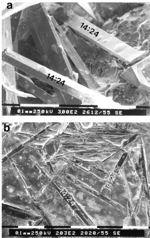
Fig. 1. SEM micrographs showing the shape of (\text{Sr,Ca})_{14}\text{Cu}_{24}\text{O}_x plates formed (a) around a pore in the sample partially-melted at 920^\circ\text{C} for 10 min, cooled down to 860^\circ\text{C} at a rate of 45 K/h, annealed at 860^\circ\text{C} for 1 h and then water-quenched and (b) at the interface between the Ag sheath and oxide compact in the sample partially-melted at 920^\circ\text{C} for 10 min and water-quenched.
