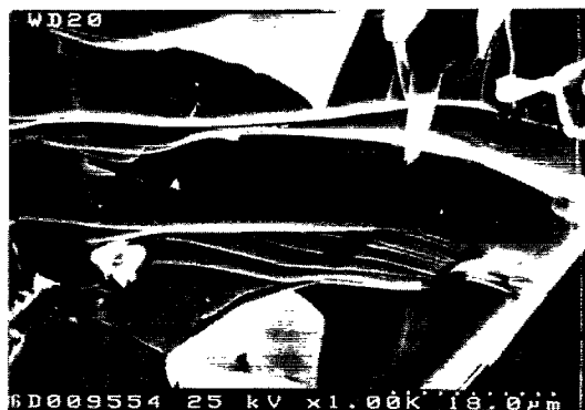
Fig. 2 The shapes of huge plate-like 2223 grains in fully-processed tape
