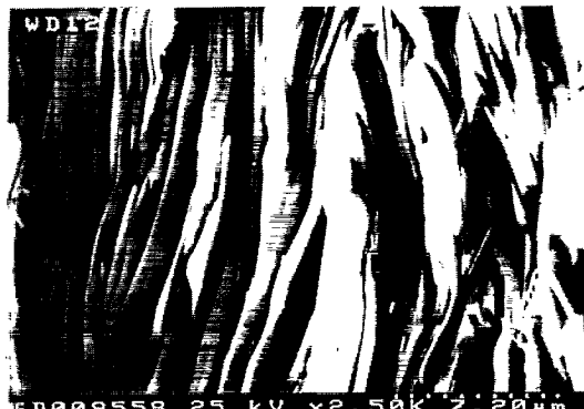
Fig. 3 SEM micrograph of a transverse fracture section of a Bi(2223) filament after the third heating cycle
