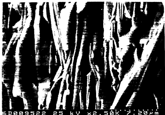
Fig. 1 Transverse fracture section of composite tape after melt processing.
