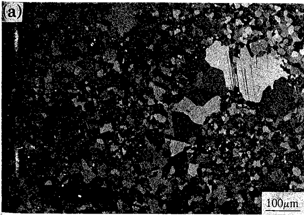
Fig. 4(a). Microstructure of specimen 3 (MTHS case) after the first annealing.
