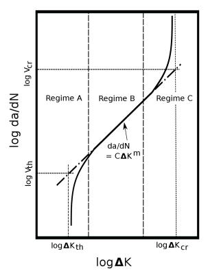
$\begin{array}{l} Regime \ A-crack \ nucleation \ and \ initiation \\ Regime \ B-crack \ growth \ or \ propagation \\ Regime \ C-sudden \ fracture \end{array}$
